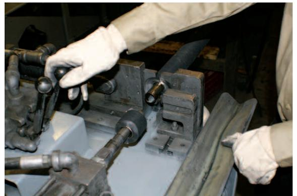
CPI extruded fins are checked for fin profile, tension, and bond, including cutting and destroying randomly selected tubes from every production run.
