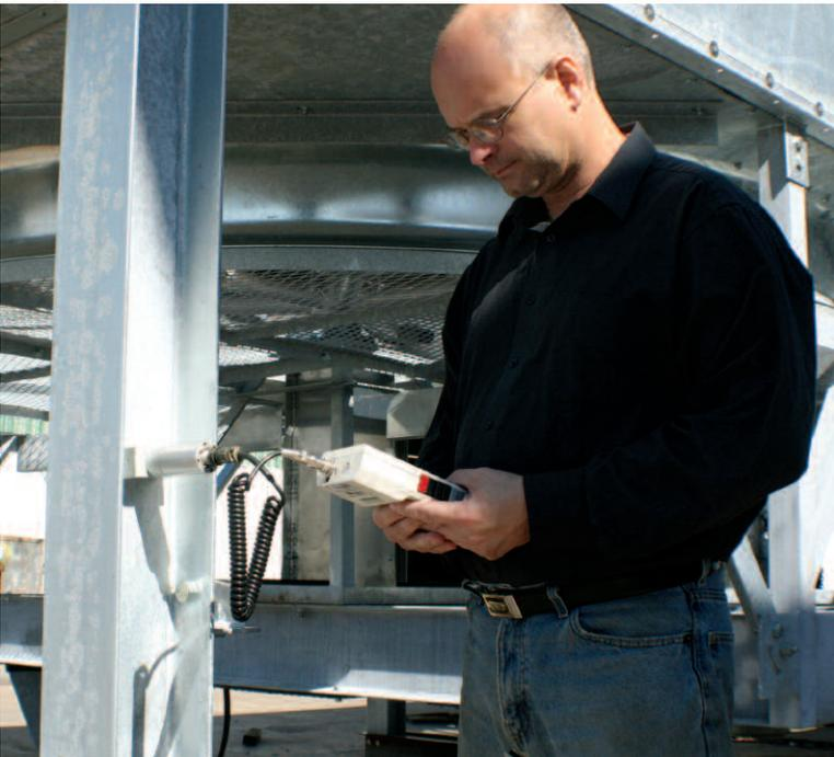
Assembled coolers are test run prior to shipment including vibration tests to API-661 (ISO 13706) standards.
