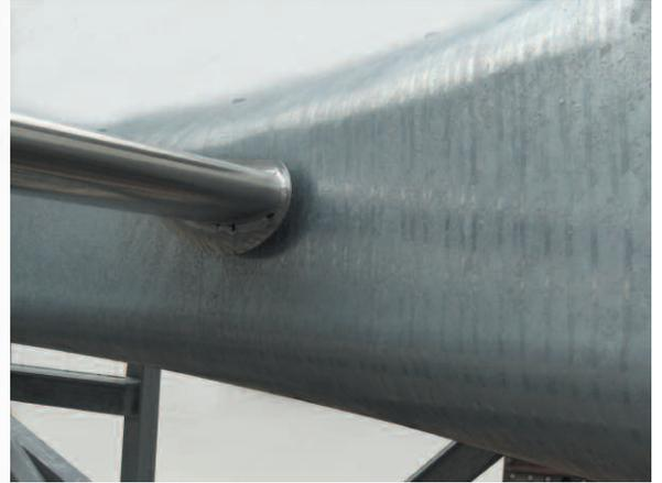
A standard CPI feature not offered by others – rounded, eased inlet and eased exit fan rings. The less abrupt change in air flow reduces static pressure, horsepower, and noise. Our fan rings, combined with other design features, allow CPI to produce some of the quietest coolers in the industry.
